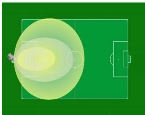
FT8 4x1000 JM Average LUX level = 20 LUX On 3800 mq area
