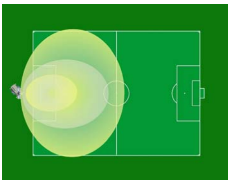
FB8 4x400 JM Average LUX level = 20 LUX On 3600 mq area
